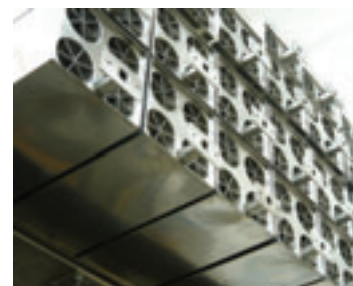
Trial Assembly of 4G-FD® Demisting Cyclones
