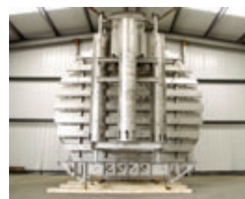
Trial Assembly of ZP-4G® Inlet Cyclones and ZHB® Distribution Baffle
