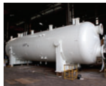
Final stage of Separator fabrication
