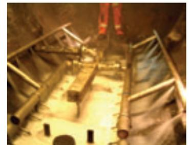
Sandwash System during Offshore Testing
